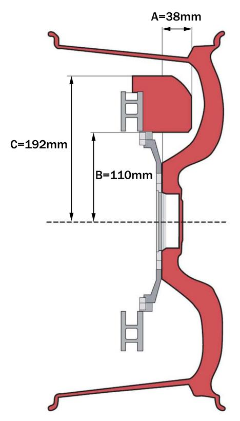
NOTE: A MINIMUM OF 2.0mm CLEARANCE MUST BE MAINTAINED BETWEEN THE WHEEL AND CALIPER IN ALL AREAS
