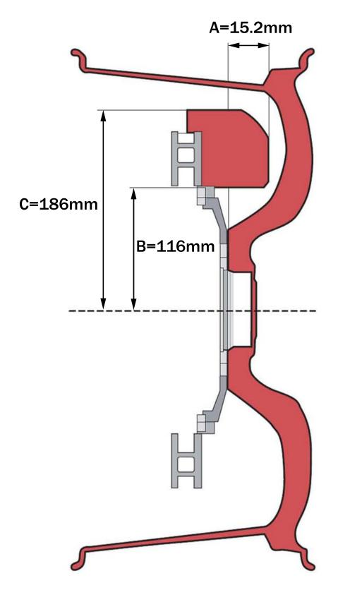
NOTE: A MINIMUM OF 2.0mm CLEARANCE MUST BE MAINTAINED BETWEEN THE WHEEL AND CLIPER IN ALL AREAS
