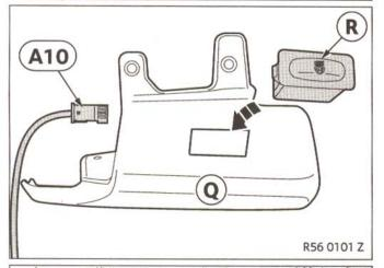
Insert button **R** as shown into the knee protection on the driver's side **Q**.
