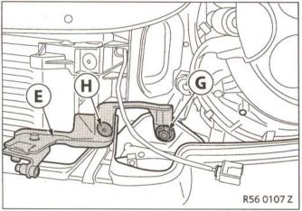
The tightening torque of hexagon nut **G** is 22 Nm. ◆
