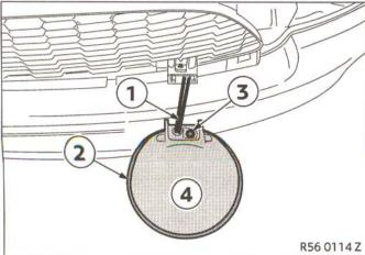
In order to avoid damaging the cable (1), hold the additional high-beam headlight (2) with one hand. ◀ Unscrew the Allen screw (3) and remove the housing (4).
