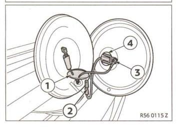
Remove the rubber cap (1) and disconnect the plug (2). Loosen the screw (3), remove it and change the bulb (4). The headlight is reassembled in the reverse order.
