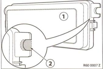
Mill out the engine compartment fuse holder (1) in the area marked (2) accordingly.
