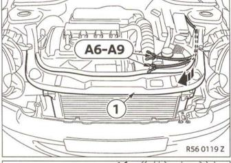
Route branches **A6–A9** along the standard wiring harness to the front end (1).
