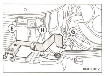
The tightening torque of hexagon nut **G** is 22 Nm. • Screw the left holder **E** using hexagon nut **G** and screw **H**.
