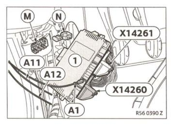
Release the footwell module (1) and socket casing X14260 (SW/GR 51-pin) (see ISTA No. 61 35 015).
