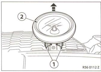
Unscrew both screws (1) and pull the additional highbeam headlight (2) carefully forwards.
