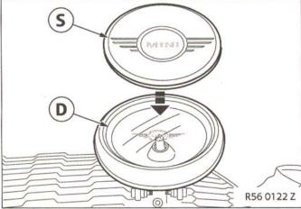
Adjust the additional high-beam headlights **D** as follows with the headlight adjustment tool:
