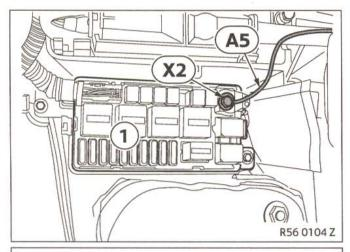
Connect branch **A5** (eyelet M8) to terminal 30 support point **X2** of engine compartment fuse holder (1).
