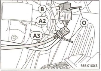
Failure to observe the instructions regarding ESD (Electrostatic Discharge) protection as per ISTA RA 61 35 ... can damage the control unit **B**. •
