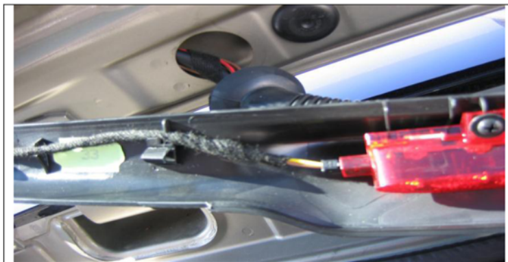
Figure 3 – Example brake light wire harness & clips
