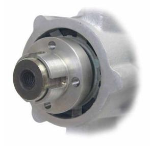
Install the pulley with front collar over the rear collar on the shaft.
