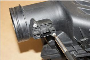
Remove MAF sensor from air filter box by removing [2] T20
