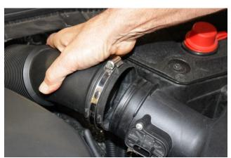
Loosen clamp at turbo inlet hose using 7mm Nut Driver and disconnect.
