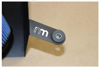
Remove metal sleeve and rubber grommet from original air filer box and install onto NM Heat Shield.
