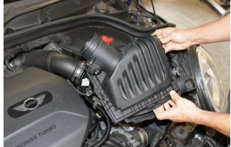
Remove the 10mm hex bolt located on driver side of air filter box then lift off. NOTE: There are [2] pin mounts that sit into rubber grommets on bottom back side, so a little effort may be required to lift air filter box off rubber mounts.
