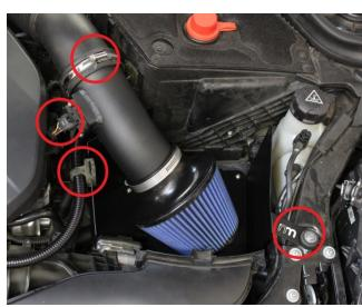
11. Install and tighten original air filter box M10 hex bolt to
