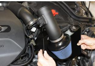
10. Install assembled NM Air Intake into lower rubber mounts
