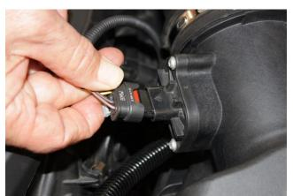
Disconnect electrical connector from MAF (Mass Air Flow) sensor. First pull outward grey tab then squeeze to release connector.
