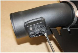
Install MAF sensor to NM Intake Pipe using supplied Philips head M4x14mm screws.
