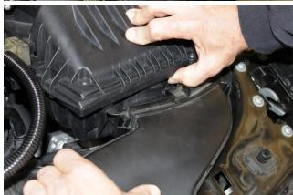
Remove the (2) 10mm nuts that hold down front air duct then push in tab at air filter box to disconnect.
