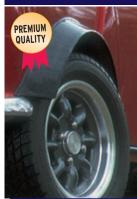
1" Wider In Fiberglass. This arch kit sticks out 2<sup>3</sup>/4" when body lines (wheel arch and moulding lip) are kept original. Arch is retained by screws through moulding
