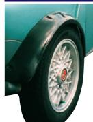
This arch kit sticks out 3" and is used when bodvline is cut awav or retained. Originally made as Group 5 Race arch where no body modifications were required, it has become a cheap 'Jack of all Trades' especially when large odd
