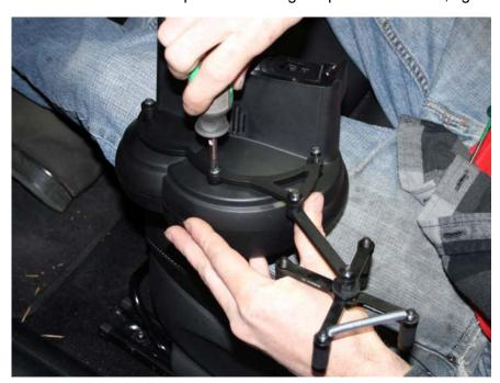
5. Re-connect the electrical clip, slide your tach back into place and put the screws on either side back into place.
