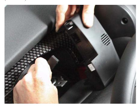
3. Remove the 3 screws (TORX) in the back of the tach.
