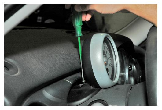
Pull the tachometer towards you to slide it off of the hidden rail. Lean the tach towards the wheel to gain access to the screws on the back of it. **Don't pull too strongly** as the wiring will stay connected.
