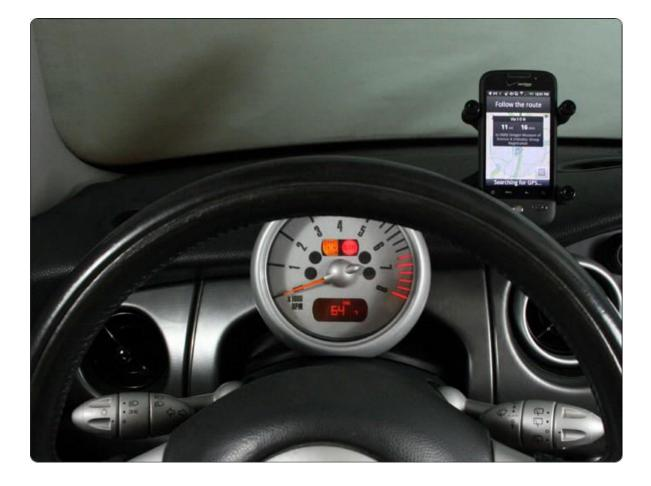
Put the tach back in its original position on the rail and reattach it with the Torx screws.
